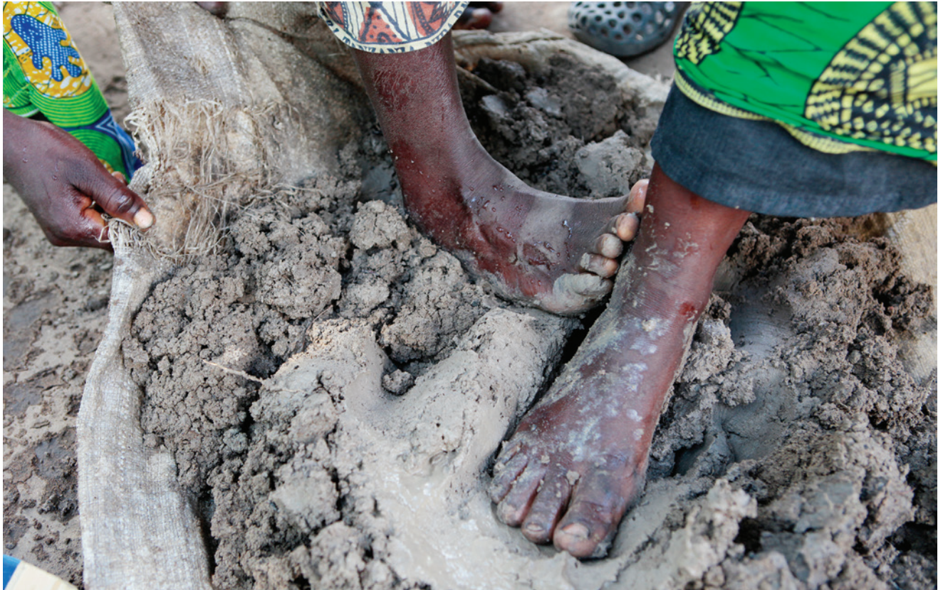
Women in Gideon village knead clay with their feet, squeezing out sticks and rocks to make efficient portable cookstoves (at right).
